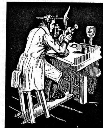
A glass engraver using a lathe operated by a foot treadle. Note the copper discs (right) of various diameters which, combined with emery moistened with oil, are used to engrave the glass. From F. Knapp Chemical Technology , Philadelphia, 1849.
